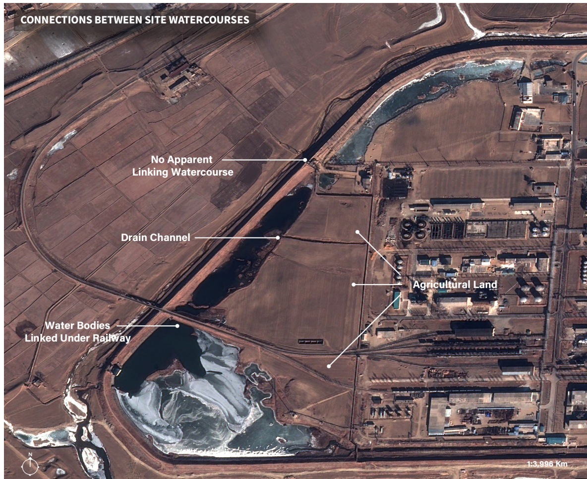
Figure 21: Connections Between Site Water Courses
