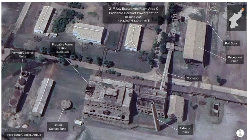
Figure 26: Area C: Probable Derelict Power Station
