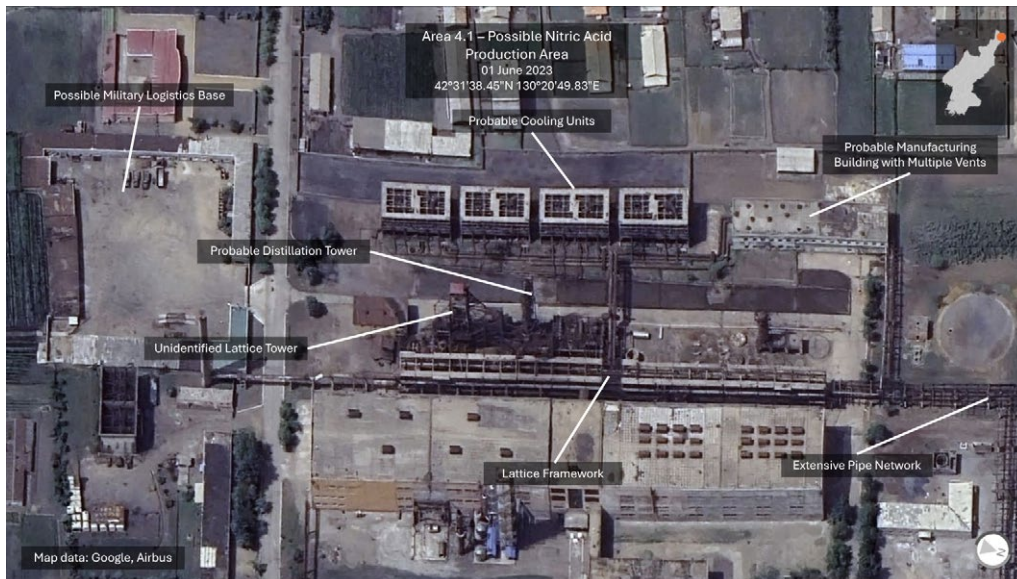
Figure 13: Area 4.1: Possible Nitric Acid Production Area
