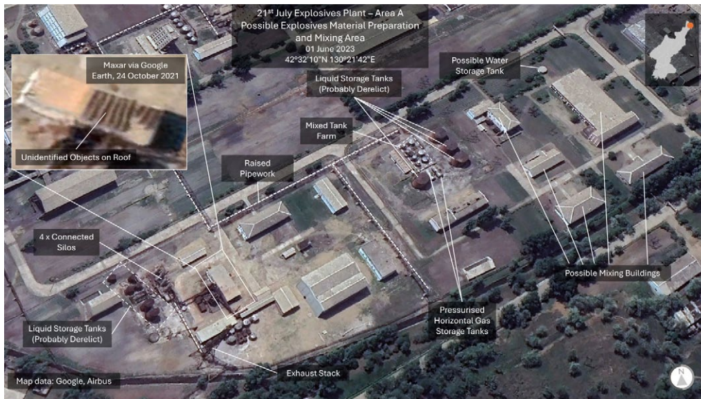
Figure 24: Area A: Possible Explosives Material Preparation and Mixing Area
