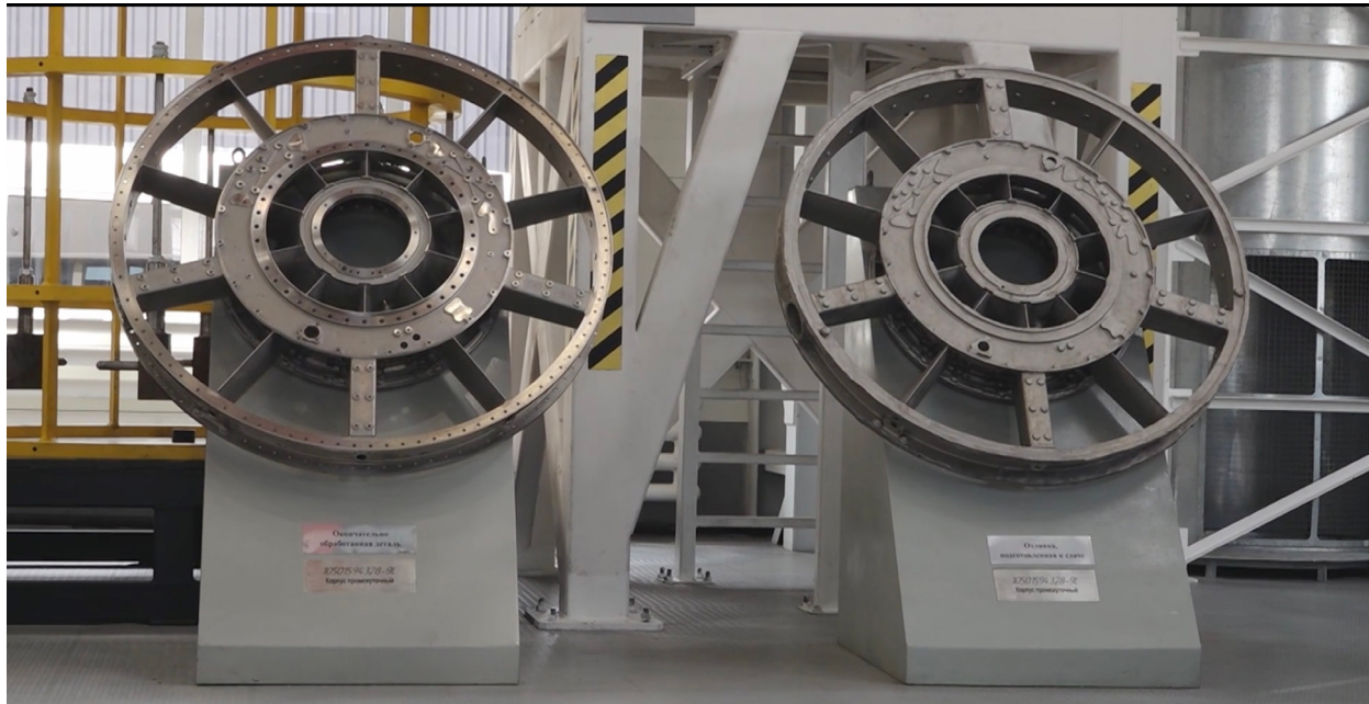
Figure 6: Intermediate Turbine Casings Before (Left) and After HIP (Right)
